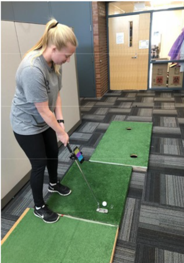
Figure 1: Experimental setup showing smartphone attached to the putter shaft and subject preparing to putt the ball to a hole (the further distance one) 6 ft away period.
