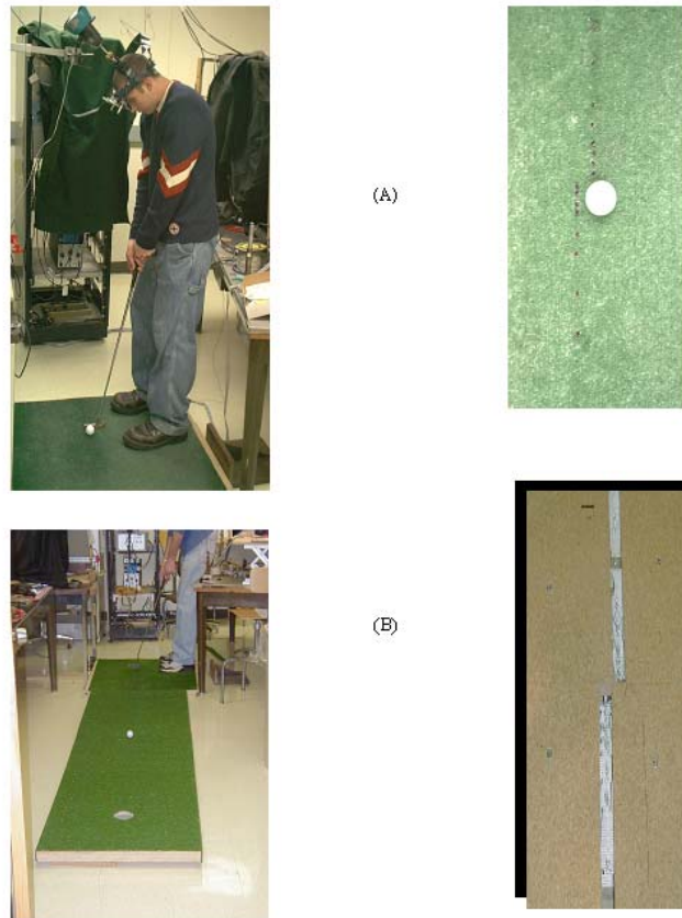
FIGURE 1. (Left column of figures) Putter platform in use during an experimental trial. (A) Subject wearing helmet (for eye and head movement measurements) and preparing to putt on the first section of the platform. Note that under this section are the embedded photodetector arrays (see Fig. 2). (B) Two other sections are combined with the first section to provide the setup for the 9-ft putts. Turning around the third section (where the hole is) and removing the middle section allows for 3-ft putts.
