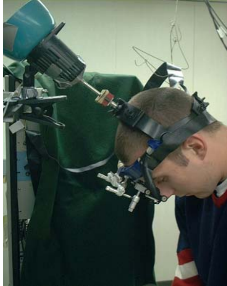
FIGURE 5. The head movement sensor is assembled by attaching the female component in the head sensor swivel unit (see Fig. 4A) to the male component in the helmet (see Fig. 4B). The swivel unit is clamped onto a frame with three directions of freedom of movement. The swivel unit itself can be pivoted and rotated about its stem. This allows for different subject heights and head angles during the putting stroke. During the experimental setup, the shaft of the potentiometer that is attached to the swivel unit (see Fig. 4A) is aligned with the head in such a way that only rotation about an imaginary axis through the top of the head and its center-of-rotation will turn the potentiometer, which in turn provides the head rotation signal.
