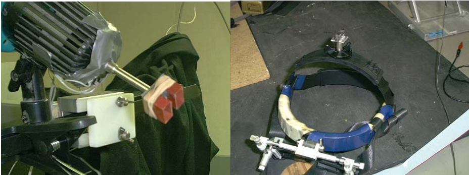
FIGURE 3. Subject wearing helmet containing the binocular eye movement sensor unit. Eye movement sensor unit in each eye contains arrays of infrared emitters (upper black rectangular piece) and detectors (lower black rectangular piece). As the eye rotates, the amount of infrared reflection from the white part of the eye changes, which can be recorded as a voltage change.
